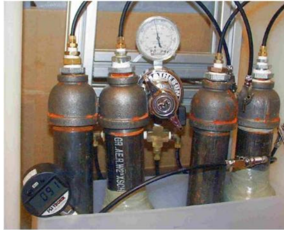
Figure 21. Supply pressure check at end of test, 1028.6 hours @ 91 psig.
