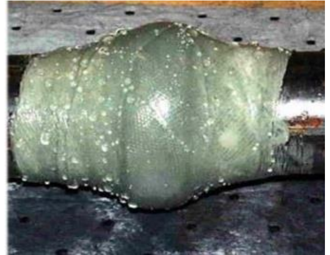
Figure 21. Supply pressure check at end of test, 1028.6 hours @ 91 psig.
